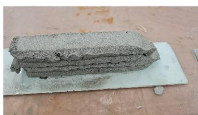
Extruded layered specimen
