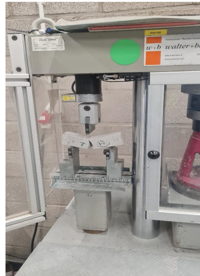
Flexural test (3-point bending) EN 12390-5
